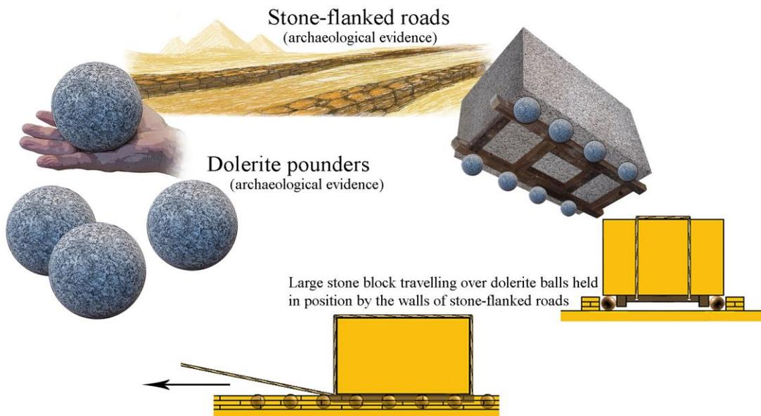
**Fig. 6. Graphic abstract of the stone ball-based transport system.**
