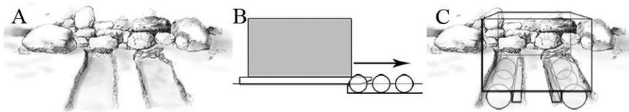
**Fig. 7. Possible system for positioning large stone blocks over dolerite balls.** A. Loading ramps channels cut into the rock at the Chephren Quarry. B-C Positioning of a block over the stone balls placed in the channels.
