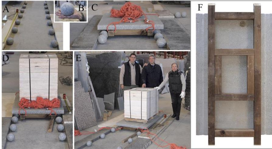
**Fig. 5. The proposed system being tested.** A. Cement 'road' and granite balls in position, ready to take the load; B. One of the granite balls (compared with those found by Arnold [Fig. 2]); C. Granite slab with the frame attached to its lower face, in position over the granite balls; D. The device, with a load of 1030 kg, ready to be moved; E. Side view of loaded device; F. View of the lower face of the granite slab showing the frame in place.
