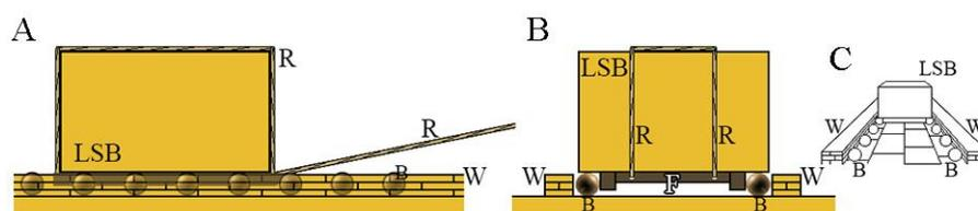
**Fig. 1. The proposed stone ball system.** A. Side view; B. Front view; C. View in perspective. B = dolerite ball; W = wall flanking road; F = Frame; LSB = large stone block; R = rope
