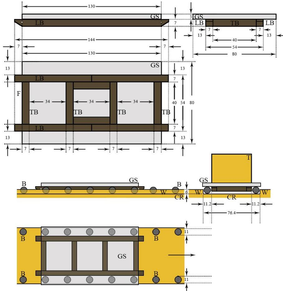
**Fig. 4. The proposed system showing the dimensions of its required components.** B = Granite ball; W = wall flanking concrete road; F = Frame; GS = granite slab. CR = concrete road; LB = lateral beam of the frame; TB = transverse beam of the frame; T = tile load. All dimensions are in centimeters.
